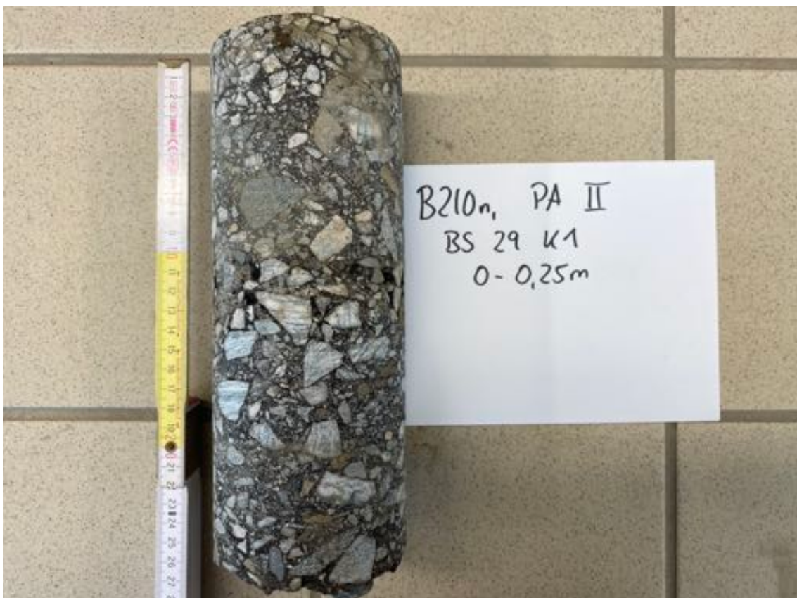
Foto 14: Asphaltkern BS 29, K 1, 0 – 25 cm
