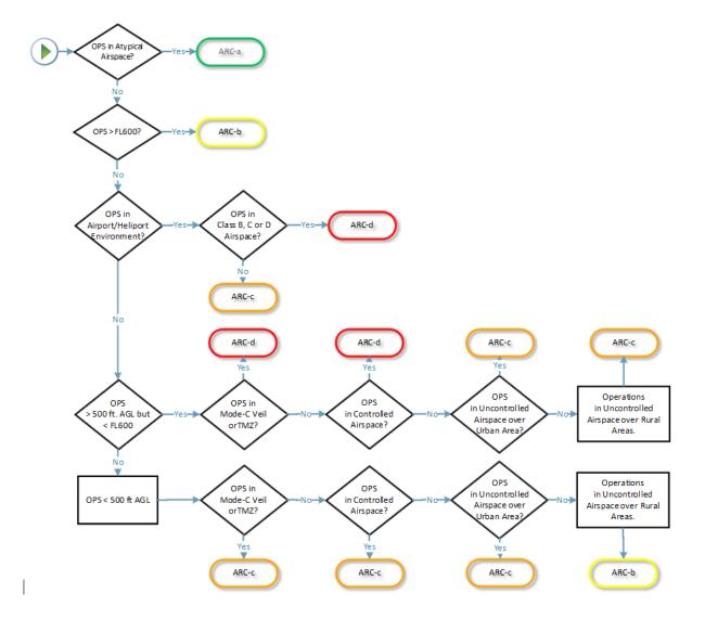
Figure 4 — ARC assignment process
